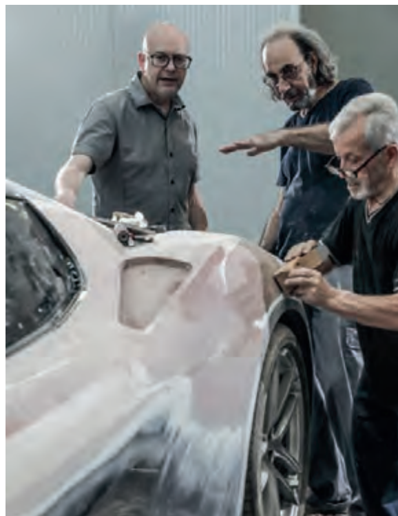
Designers and clay modellers finesse the final shape of the vehicle's distinctive wheel arches and nose.
